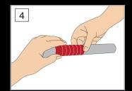
To complete wrapping of object, wrap SPITA ResQ-tape completely over previous layer and press firmly.
