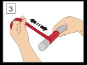
While holding SPITA ResQ-tape in place, begin STRETCHING at 3 to 4 times it's length and wrap object with 50% overlap to ensure a proper seal.
